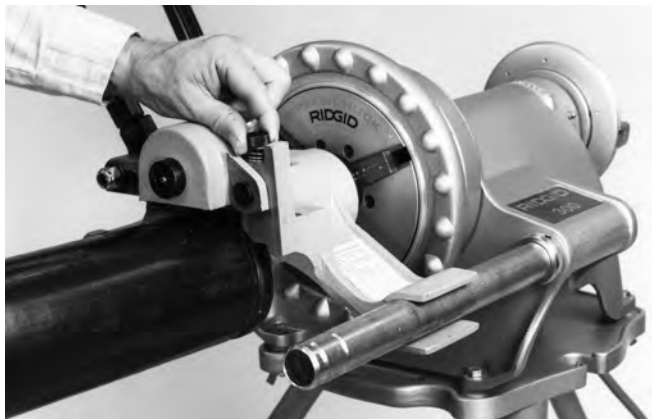
Figure 11 – Tighten Depth Adjustment Screw
