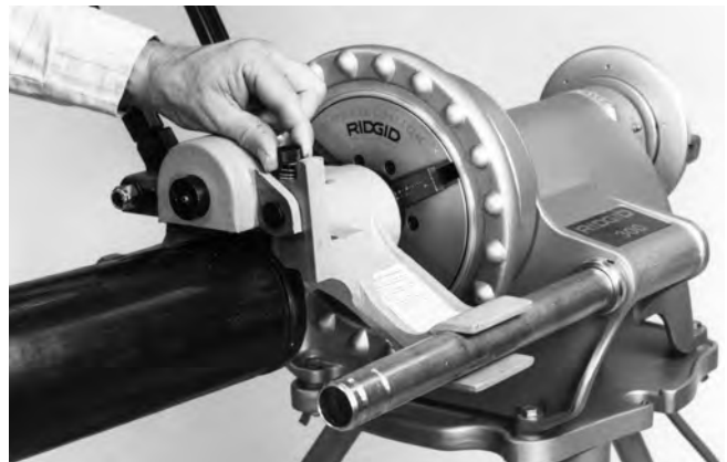
Figure 10 – Loosen Depth Adjustment Screw
