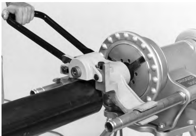
Figure 12 – Forming the Roll Groove
