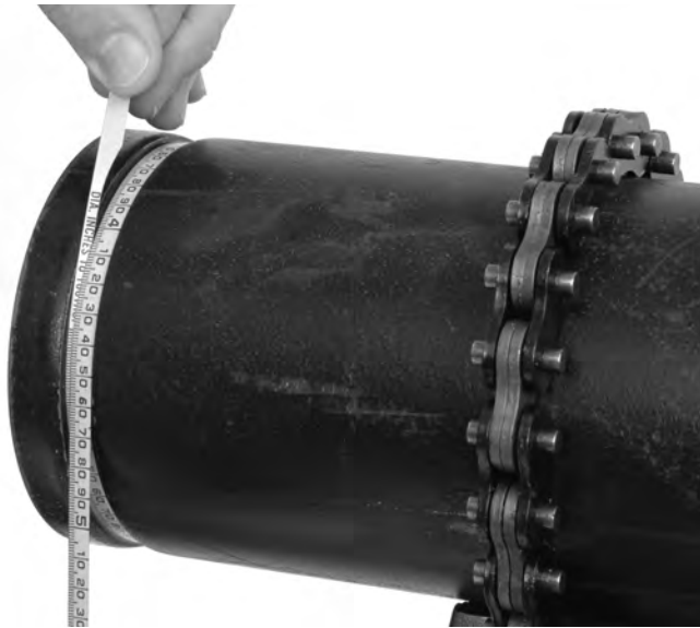
Figure 21 – Checking Groove Diameter with a Diameter Tape
