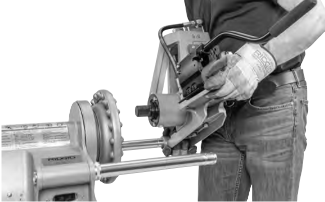
Figure 7A – Installing 918 on 300 Power Drive
