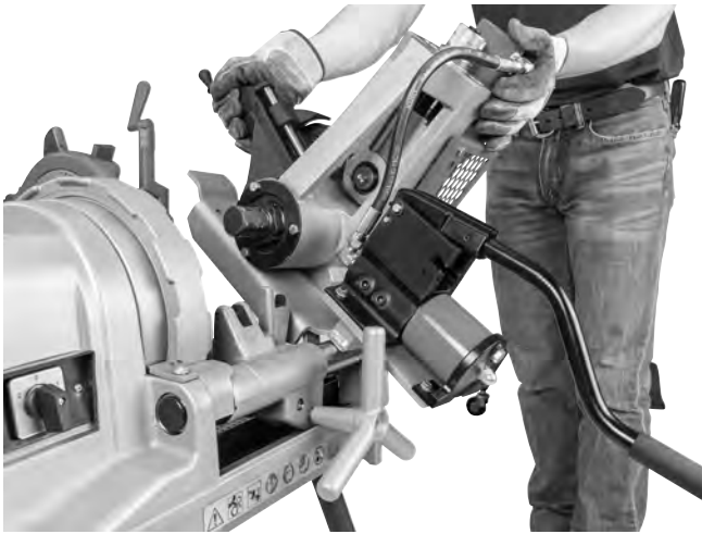
Figure 8B – Installing 918 on 1233 Threading Machine
