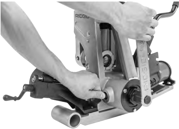
Figure 28 – Engaging Spindle Lock and Loosen Draw Bolt
