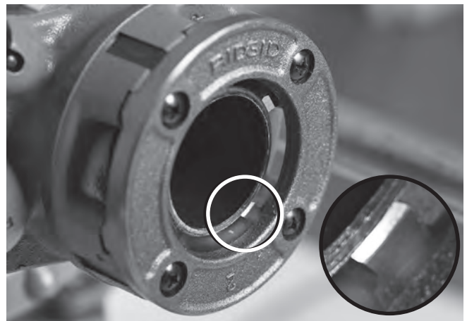
Figure 19 – Pipe Even with Edge of Dies
