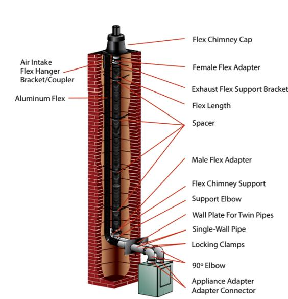
Flex Through Chimney w/ Air Intake
