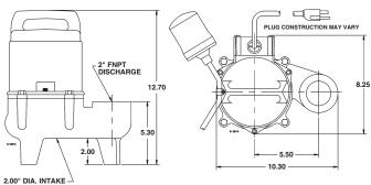
\*Note: Mechanical Float Switch to be installed by customer. Installation at 3.5" tether length float switch will activate pump at 15"-17" on level and 8"-10" off level.
