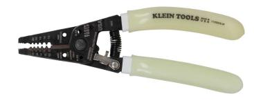
Klein Tools' High-Visibility Wire Stripper / Cutter allows you to find your tools in the dark. The glow-in-the-dark grips can stay illuminated for up to 30 minutes. Plus, they charge in natural or artificial lighting. This Wire Stripper and Wire Cutter tool cuts, strips, and loops 10-18 AWG Solid and 12-20 AWG Stranded wire.
