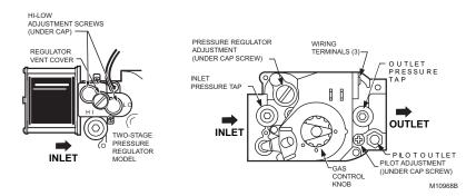
Fig. 6. Top view of gas control.
