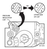
Fig. 1. Top view of convertible pressure regulator cap.
