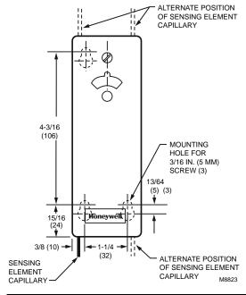
Aquastat® Controllers are immersion type devices for limiting or regulating the temperature of liquids in boilers, storage tanks, and other applications where temperature control is required.
