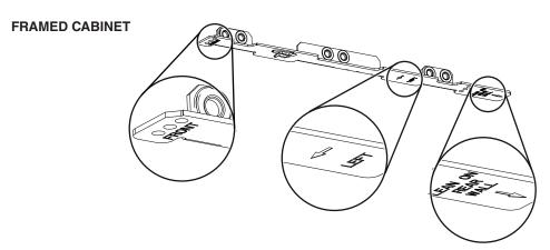
Refer to the marking on brackets to determine the correct installation side and orientation.
