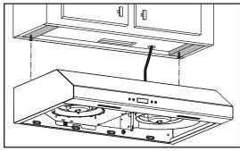
3] Secure the hood to the cabinet using two (2) no. 8 x 5/8" round head wood screws (included in parts bag). Insert one (1) screw per side, in the slots (as shown below). Attach power cable to the hood using the strain relief.
