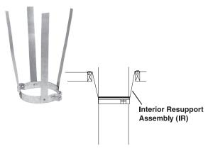
**NOTE:** 4" IOS is not exactly as shown. The 4" IOS is installed immediately on the section of chimney above the upper elbow of an offset and will support 25' of chimney.
