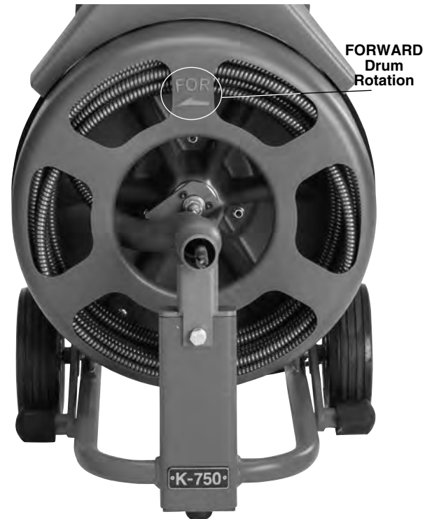
Figure 6 – Proper Drum Rotation (FOR Switch Position)
