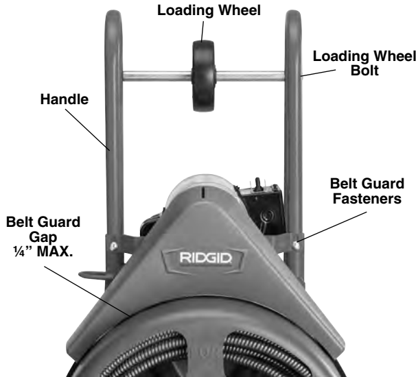
Figure 3 – Handle Installation and Belt Guard Adjustment
