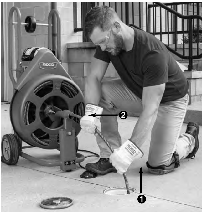
Figure 13 – (1) Pulling Cable and (2) Feeding into the Drum
