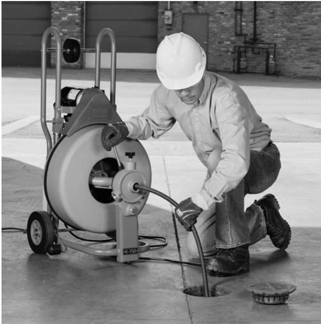
Figure 14 – Operating the K-750 using the AUTOFEED
