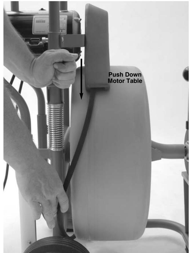
Figure 17 – Releasing Belt Tension
