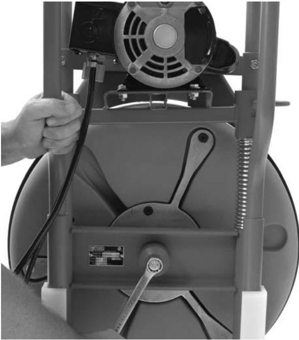
Figure 18 – Removing Drum Bolt
