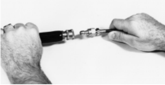
Figure 3 – Connect jetter hose to jetter
