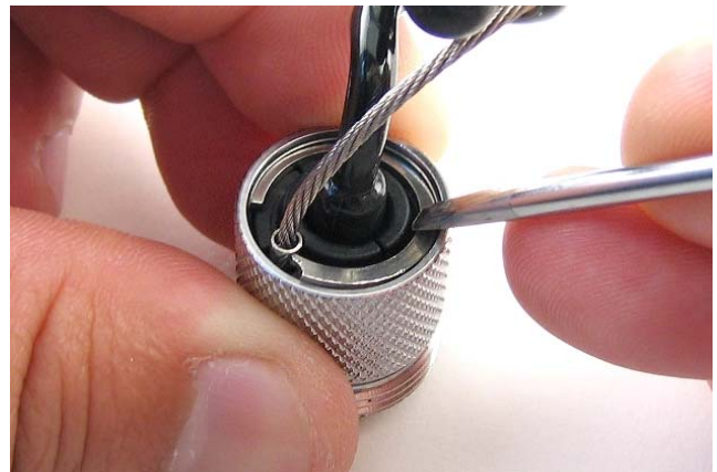
Insert the retaining ring in the back of the locking sleeve. If necessary, use a flat blade screwdriver to complete the installation.
