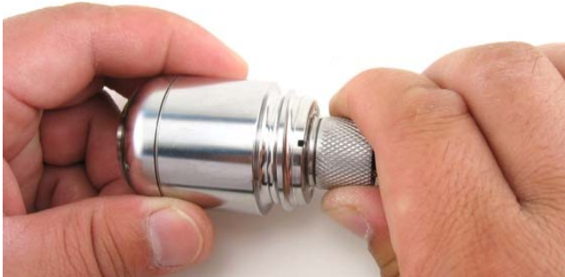
Unscrew the locking sleeve from the back of the camera head and slide it back to expose the connector.
