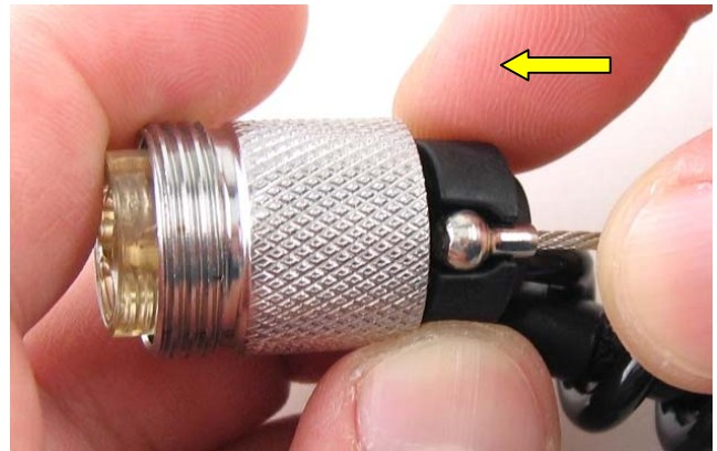
Place the safety cable in the groove on the slotted insert and push the two inserts and safety cable ball into the back of the locking sleeve.
