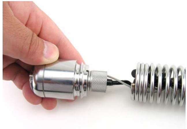
Back-twist the camera head to counteract the twisting that will occur when the camera head is threaded onto the spring. See Figure 2.
