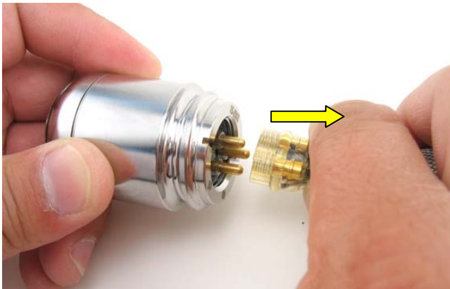
Unplug the connector at the back of the camera head.
