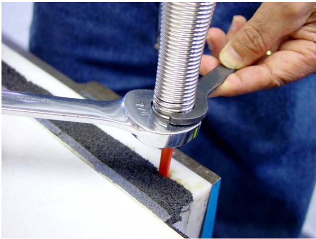
If you are replacing the Flexmitter on the Compact, hold the rear spring shell with a 7/8" wrench and use the old style metal spanner for the mini to unscrew the spring.
