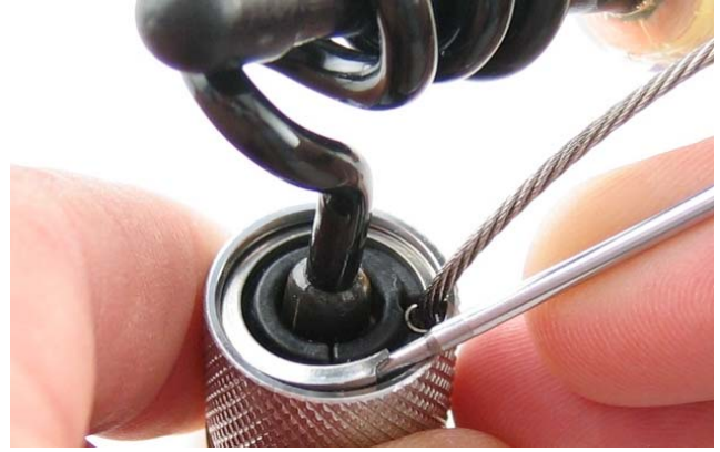
Use a fine point flat blade screwdriver to remove the retaining ring, then pull the safety cable & inserts free from the back of the locking sleeve.
