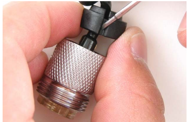
Insert a flat blade screwdriver in between the inserts and twist to separate them. Set them aside for use during assembly.
