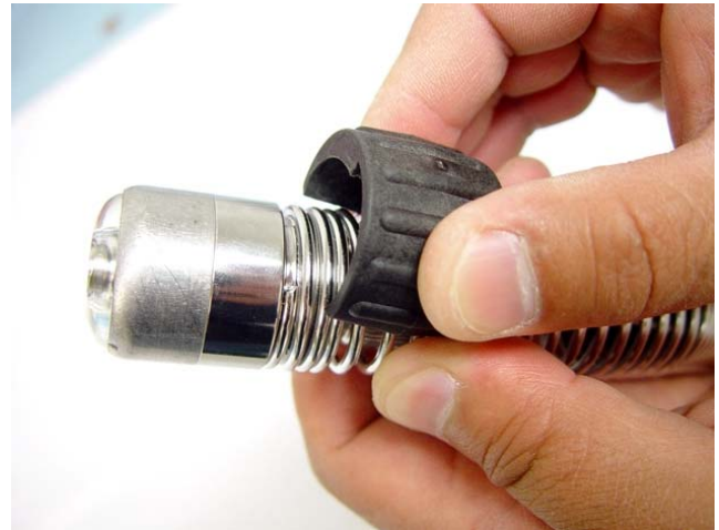
To remove the camera head, align the tab on the spanner wrench with the end of the spring and snap the wrench into (see Figure 1).
