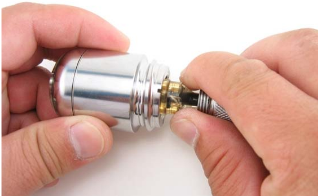
Plug the Flexmitter connector into the back of the camera head.
