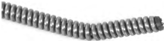
Figure 15 – Bend At Cable End
