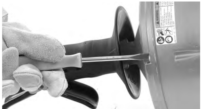
Figure 13 – Loosen 4 Drum Screws About 3 Full Turns, But Do Not Remove
