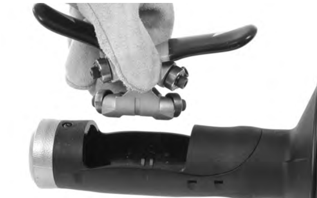
Figure 12B – Removing AUTOFEED Mechanism From Housing
