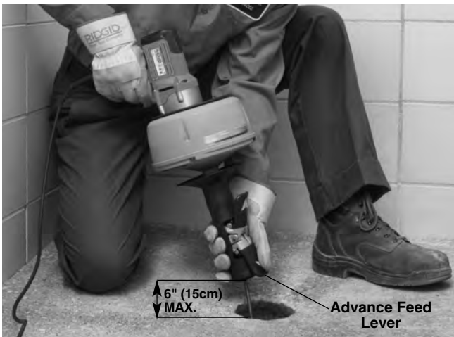
Figure 10 – Feeding Cable With AUTOFEED
