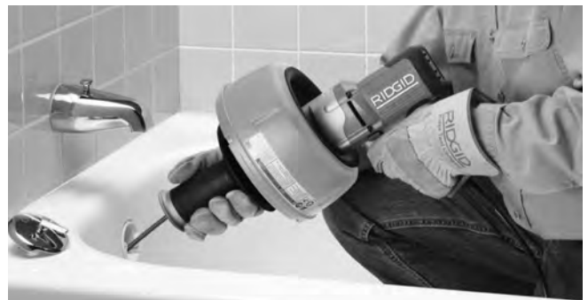
Figure 9 – Push Cable Down Drain Line
