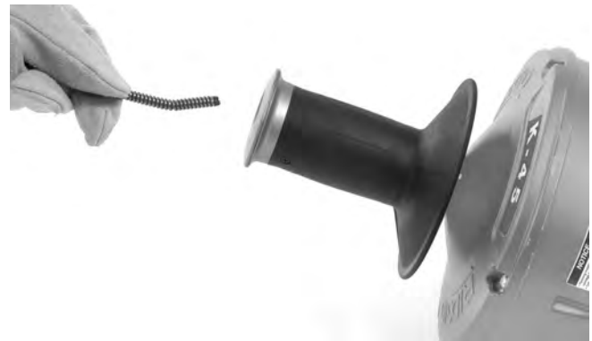
Figure 17 – Loading Cable Without Changing Inner Drum
