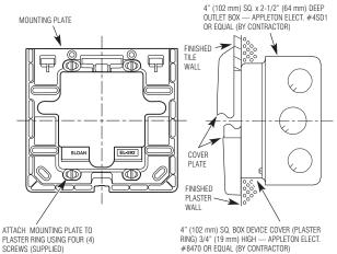
To ensure a perfect rough-in, Sloan recommends the use of the EL-485-A Flushometer electrical box positioning and support kit. Specify and order the EL-485-A kit separately. Consult factory for installation details.
