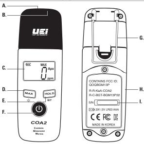
A. CO Sensor Vent: For sensing CO levels (keep clear of obstructions).
