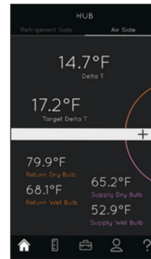
Air Side displays return & supply measurements.
