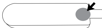
Apply a small area of thermal compound to the back of the sensor case where shown
