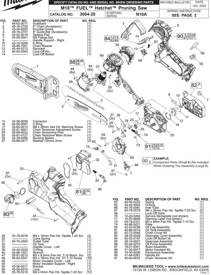
As an aid to reassembly, take notice of wire routings and position in wire guides and traps while dismantling tool.
