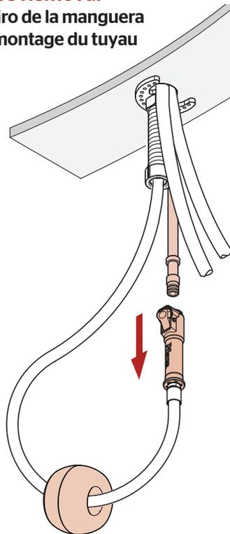
**To remove hose, press on the tabs and pull hose connector down.**
