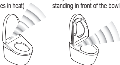
Body sensor A (Detects changes in heat)
