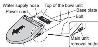
**3** Clean the top of the bowl unit and the bottom of the main unit.
