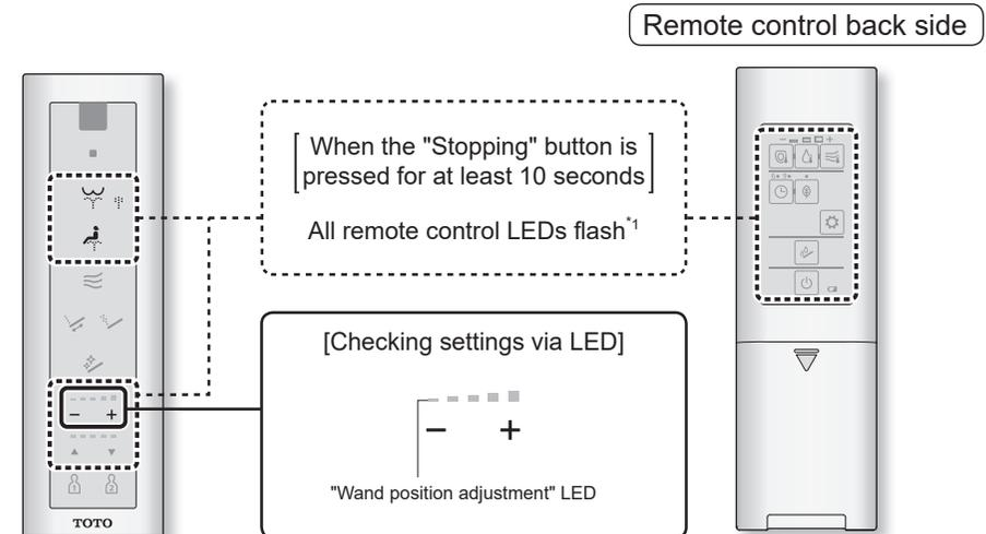
\*1 During setting, if the next button is not pressed within about 60 seconds, the light will stop flashing. If you fail to complete the setting, redo from the step 1.
