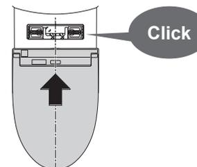
Align the main unit with the center of the base plate and press it firmly onto the base plate until a click sound is heard.
