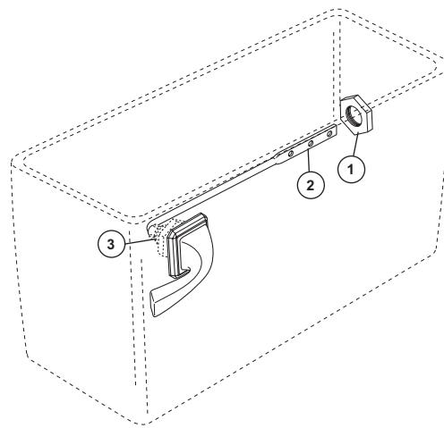
Orient handle assembly as shown. Slide mounting nut (1) over shaft (2). Move the nut to the handle assembly and tighten onto the threaded mounting shaft (3).
