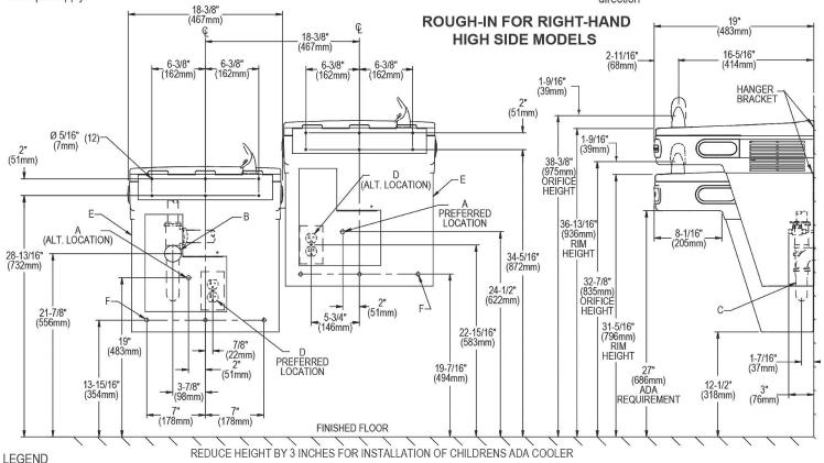
A = Recommended water supply location. Shut off valve (not furnished) to accept 3/8" O.D. unplated copper tube connect. Up to 3" (76mm) maximum out from wall. B = Recommended waste outlet location. To accomodate 1-1/2" nominal drain. Drain stub 2" (51mm) out form wall.
