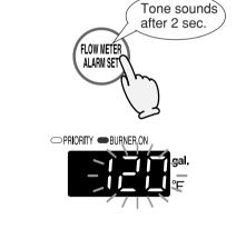
Change the temperature using the setting buttons.
