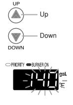
The upper limit of the hotwater supply temperature can be changed to 100°F, 105°F, 110°F, 115°F, 120°F, 125°F, 130°F, 135°F or 140°F.
