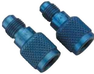
Liquid charging is recommended when charging blends into refrigeration and air conditioning systems. A liquid charging adapter is necessary for safe and fast liquid (saturated vapor) charging through the low pressure side of a system. The YELLOW JACKET liquid charging adapter connects to the cylinder valve or refrigerant tank.
