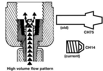
The patented “Adjust-a-Valve” reaches out-of-tolerance Schrader valves in 1/4", 3/16" and 5/16" couplers. Simply rotate the opener with needle nose pliers to the desired height and when finished, rotate it back. “Adjust-a-Valve” for 1/4" and 5/16" hoses is the same.
