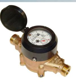
earth magnets eliminate slipping and uncoupling to increase overall accuracy. The magnet is connected to a gear train which translates the impeller's rotation into volume totalization displayed on the register dial face.
