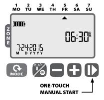
With the controller in AUTO RUN mode, press and hold | for 3 seconds to begin watering all zones that have a programmed runtime.
