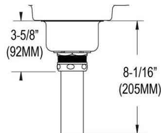
Sink with Drain Kit Installed
