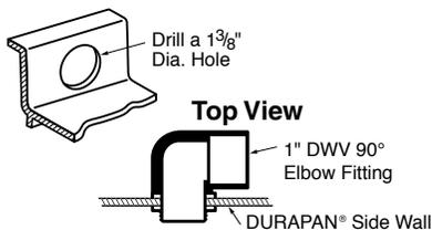
Drill hole through any side or back wall. Install solvent weld elbow fitting and connect 1" PVC pipe (not provided) leading to DWV drain.
