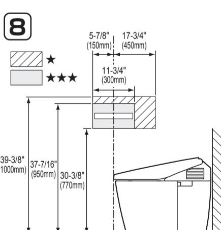
9 Temporarily place the remote control in the position determined in 8 and confirm the signal reception of A-1.
