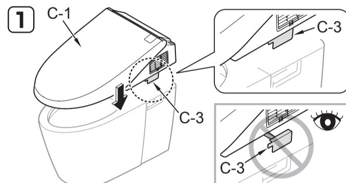
How to remove "C-1" when it is placed temporarily.
