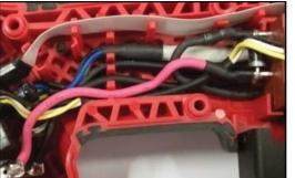
Carefully place/route ribbon cable in traps as shown.
