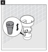
Turn bottom screw counter -clockwise to adjust unit up and down.
