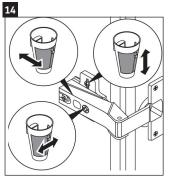
The top screw will adjust up and down, back screw will adjust closer and further, from the cabinet, fron screw will adjust left and right.
