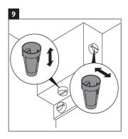
Check the screws which allow adjustment of the unit. The top screw will adjust front to back and the bottom screw will adjust up and down.
