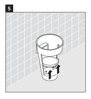
Lift the unit up and onto the mounting screws.
