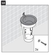
Using three screws and three washers secure the washbasin to the vanity.
