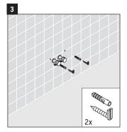
The plastic anchors provided are for concrete wall applications. For wood stud walls bolts should be screwed into wood backing.
