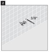
Using 3/8" drill bit, drill the anchor holes that have been marked.
