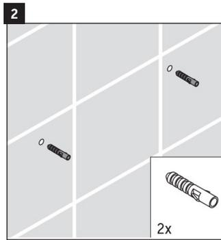
Drill the anchor holes that have been marked. The Plastic anchors provided are for concrete wall applications. Insert plastic anchors into the holes.
