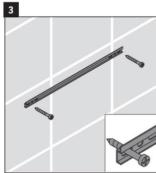
Screw the bracket(s) to the wall the specified locations. For wood stud walls, bolts should be screwed into wood backing.
