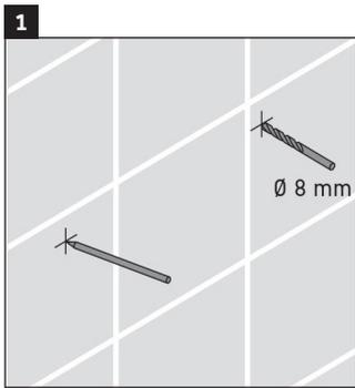
Reference the cabinet specification to establish the position of mounting bolts, mark the holes to be drilled for the anchors.
