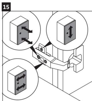
The top screw will adjust up and down. Back screw will adjust closer and further. From the cabinet and front screw will adjust left and right.
