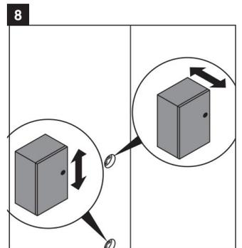
Check the screws which allow adjustment of the unit. The top screw will adjust front to back and the bottom screw will adjust up and down. Make adjustments to the level as needed.
