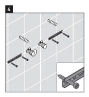
For wood stud walls, bolts should be screwed into wood backing.
