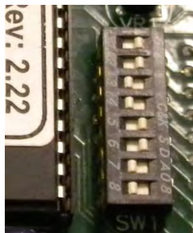
View of the Dip Switch set for normal mode.
