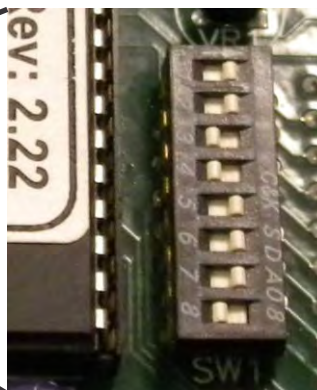
Close up view of the Dip Switch set for calibration mode
