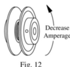
safety. Adjust pulley to a larger diameter and readjust belt tension, plug motor in, install pad frame, and retest amperage draw. Repeat this process until correct amperage draw is attained. Increasing motor pulley diameter increases amperage draw. Decreasing motor pulley diameter decreases amperage draw (see Fig. 12).
