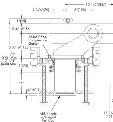
Options (Select One or More) Suffix Description 3" No Hub Fitting -3 -36 36" Long Barrel Fitting -CA-100-EXT Aux. Support System w/Extended Nipple ABS Extended Nipple (Up to 24") -M3 Galvanized Steel Nipple 7" -M11 Tiling Frame -M20 Flush Valve Supplort
