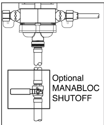
Local code may also require the installation of a check valve, PRV (pressure reducing valve), back flow preventer, etc. To prevent debris and other particles from entering the system, a strainer may be installed in the service line.
