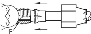
Holding the tube so that it does not back out of the fitting, slide the white Lock-In insert and ferrule snugly against the chamfer inside the port socket.
