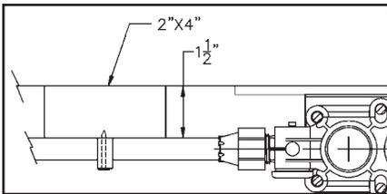
Use one clamp per tube to ensure that the tubing is held securely. Clamps shall be positioned NO FURTHER than six (6) inches from the end of the port. DO NOT pull tubing tight. Leave at least 7" of slack per 50' of tubing run.
