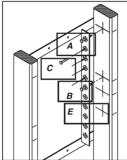
11. Using an awl, nail, or other pointed tool (C) mark the stud by tapping through the Drill Guide at each printed center line between the two nails. Carefully remove the Drill Guide. If the MANABLOC does not have a divider plate, go to step 13.
