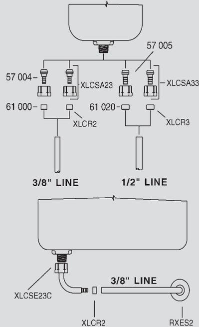
Tighten fixture nut hand tight plus an additional 1/4 turn. Check all connections for leaks.
