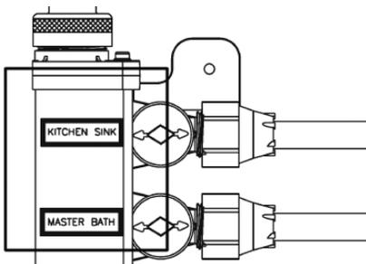
*Self-adhesive labels are supplied with the MANABLOC. Tubes pulled as a bundle, or those not connected immediately, should be marked at both ends with a permanent marker designating the fixture supplied.*
