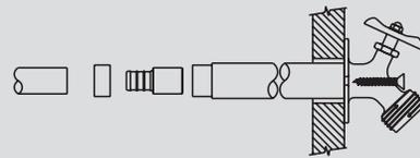
Hose bibbs supported by the structure can be connected directly.
