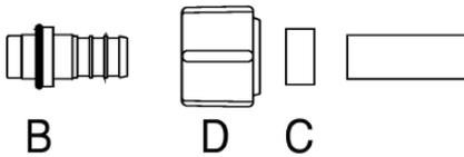
Insert the brass adapter (B) fully into the end of the tubing as shown.
