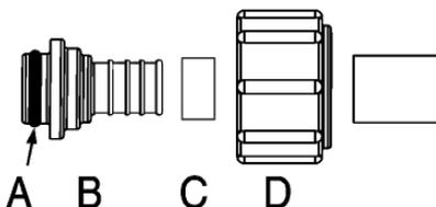
Insert the barbed end of the fitting (B) fully into the end of the tubing as shown.
