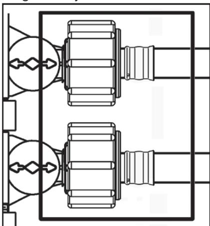
5. Open the port valve(s) before turning on the main water supply.
