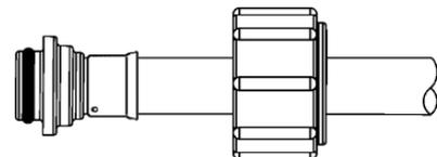
2. Check full tubing insertion at view hole of sleeve, then press the sleeve with an appropriately sized press tool. See section 5 from the PureFlow installation manual for pressing instructions.
