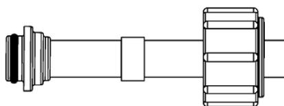
2. Insuring sealing element (A) is in place, insert the fitting into the desired port until the fitting flange sets flush with the end of the port.
