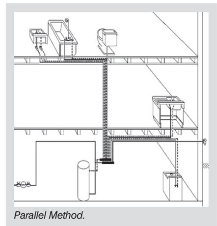
as well as eliminating interference between fixtures. Often each fixture can be fed with smaller diameter tubing which is easier and faster to install.
