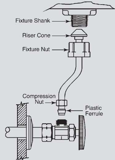
Thread fixture nut onto fixture shank. Tighten fixture nut hand tight plus an additional 1/2 turn. Slide compression nut and supplied plastic ferrule over tube as shown. The long taper of the ferrule goes towards valve. Tighten compression nut according to valve manufacturer's recommendations.
