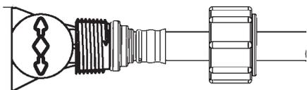
4. Slide the swivel nut (D) over the press sleeve (C) and thread the nut onto the MANABLOC port, hand tighten only.
