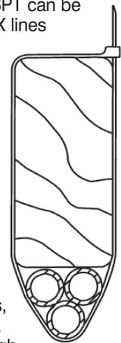
8. Holes drilled through studs, joists, plates, headers, etc. must be large enough to accommodate tubing bundles without binding, to allow free movement. Several smaller holes (accommodating a few lines each) may be preferable to drilling a bundle-size hole. In no case should the hole size exceed building code guidelines, as this could weaken the structural support members.
