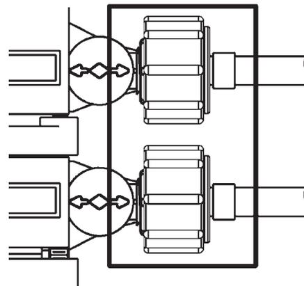
5. Open the port valve(s) before turning on the main water supply.
