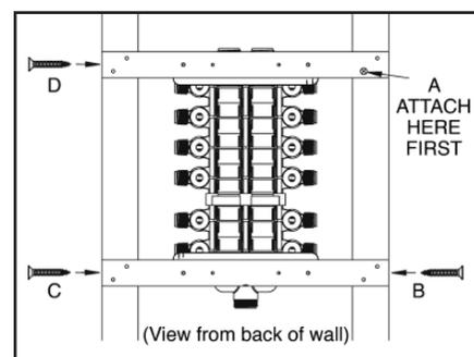
4. Line up the LOWER Mounting Strap with the back outer edge of the stud and attach it in the same manner (B). Attach the remaining strap ends (C & D) to the other stud, and tighten all screws.
