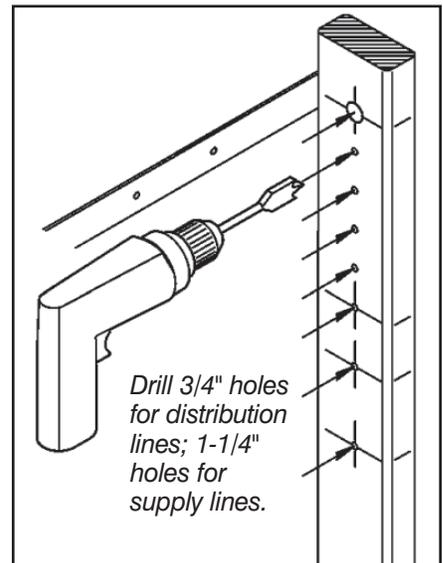
15. Mark and drill any holes for main water supply and hot water supply/return lines at this time. An 1-1/4" bit will provide adequate clearance for 3/4" or 1" tubing. The tubing shall enter and/or exit the MANABLOC in a straight line
