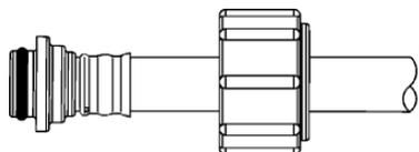
3. Insuring sealing element (A) is in place, insert the fitting into the desired port until the fitting flange sets flush with the end of the port.
