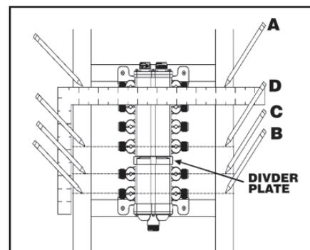
Mark the centers of the top and bottom MANABLOC ports (A, B) and the ports directly above and below any divider plate (C, D)
