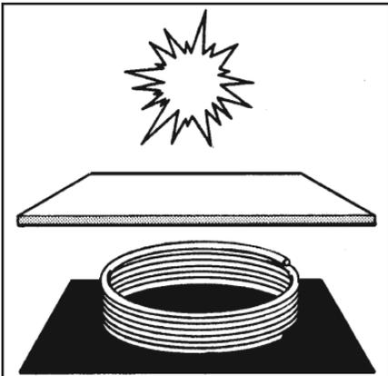
PEX tubing should always be shielded from direct or indirect sunlight.
