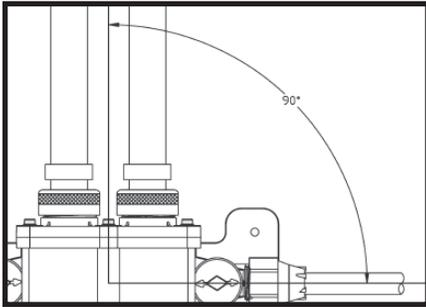
7. When attaching the distribution line tubing to the 2 x 4 supports, be sure to use appropriately-sized Viega tubing clamps (For example, use stock code 52 000 for 3/8" tubing and stock code 52 020 for 1/2" tubing).
