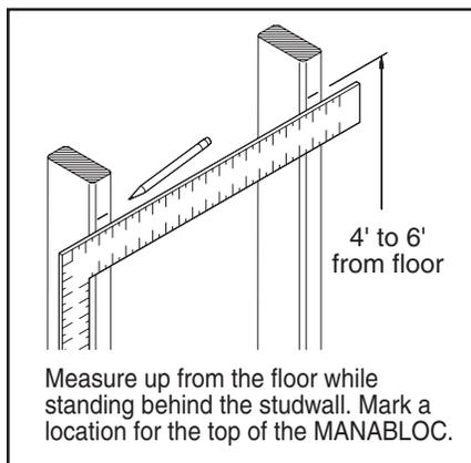
This mark should be between 4 feet and 6 feet from the floor but may be at any height, provided the height will allow all valves on the MANABLOC to be accessible. With a framing square or level, transfer and mark the noted height on the other stud.
