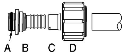
Insert the barbed end of the fitting (B) fully into the end of the tubing as shown.
