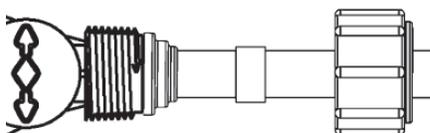
3. Slide the crimp ring (C) to within 1/8" to 1/4" from the end of tube. Crimp the ring with an appropriately sized full-circle crimp tool.
