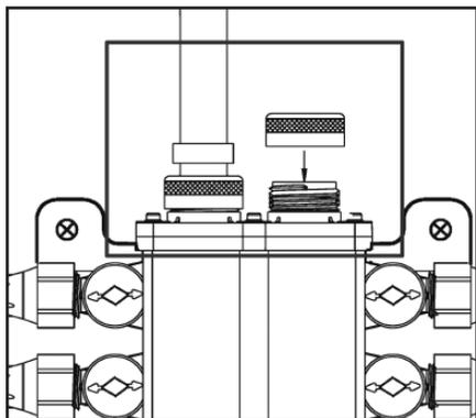
If a main inlet/outlet will not be used, it must be capped (use Part No. ECAP1).
