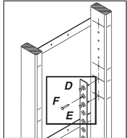
14. Drill 3/4" holes through both studs at each marked location. Be sure to hold the drill level and perpendicular to the stud to prevent drilling holes at an angle. Remove any splinters or burrs made during drilling.
