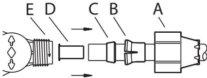
The long taper of a 3/8" ferrule (C) must be TOWARD THE END OF THE TUBE; a 1/2" ferrule is symmetrical and may be installed facing either direction. Insert the stainless steel stiffener (D) COMPLETELY into the end of the tubing.
