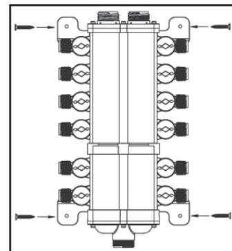
6. As the distribution lines are connected to the MANABLOC (see section 6), ensure that the tubing exits the unit at a 90 degree angle to the centerline of the MANABLOC so as not to induce bending stress on the MANABLOC.
