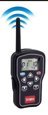
For simple time saving operation of zones and schedules, Toro® introduces the Smart Connect® Handheld Remote. The remote works with the EVOLUTION® Series Controller to activate zones and schedules from up to 1000' line of sight distances.
