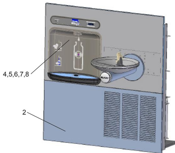
**Figure 8 – Lower Panel Installation**
