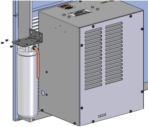
**Figure 4 – LZWS-ERP8-RF Filter Mounting
