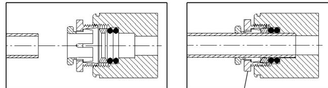
Note: Screw the locknut hand tight to seal
