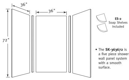
Designed to fit base areas 36" deep or smaller x 36" wide x 72" high or smaller (914 mm x 914 mm x 1829 mm)
