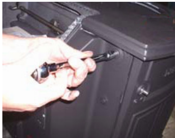
Fig. 4 Remove 4 Upper Fireback Bolts (Rear of 1945 Model)
