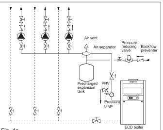
Fig. 4a Multi-zone system using zone pumps. Piping arrangement for best air elimination (see note on following page)
