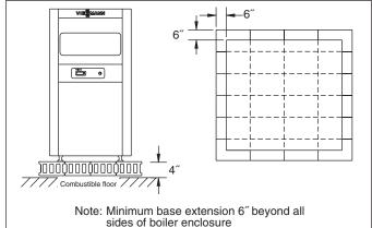
Fig. 3 Suggested base for installation on combustible floor
