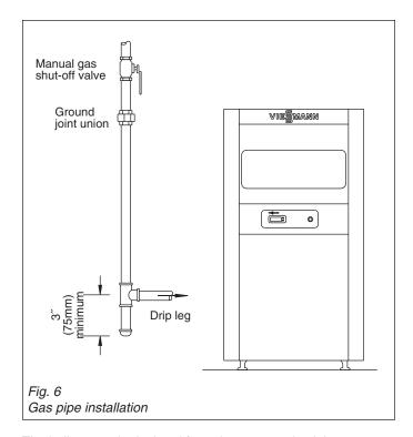
The boiler must be isolated from the gas supply piping system by closing its individual manual shut-off valve during any pressure testing of the gas supply piping system at a test pressure equal to or less than  $\frac{1}{2}$  psig (3.5 kPa).
