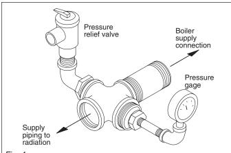
Fig. 4 Pressure relief valve installation (Use fittings supplied in accessory pack)
