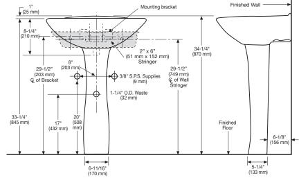
NOTE: Rough-in measurements may vary 1/4" (6.4 mm ±). NOTE: For installation of waste outlet through-the-floor, an S-trap is required.
