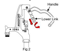
If the Handle does not "snap" closed approximately 3" from the head casting upon turning off the hydrant, follow the instructions to adjust the linkage and handle tension.
