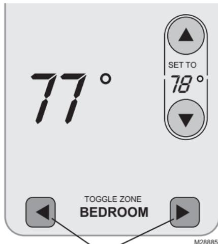
If you have multiple thermostats Temperature is measured at each thermostat. Press **TOGGLE ZONE** buttons to choose which room to display and adjust (see page 7).
