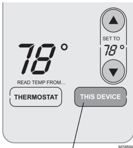
If you have only one thermostat Temperature is measured at thermostat or remote control, as you choose. You can move the remote control as needed, so the room you are using maintains a comfortable temperature (see page 6).
