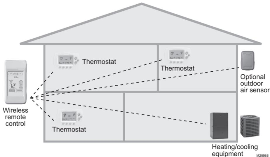
If you have one thermostat, you can move the remote control around your home (like a mobile thermostat) to make sure the temperature is comfortable in the room you're using.
