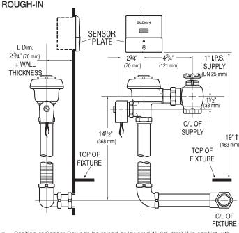
Position of Sensor Box can be raised or lowered 1" (25 mm) if in conflict with Handicap Grab Bars.
