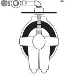
3. When the user steps away from the OPTIMA Sensor, the circuit waits 3 seconds (to prevent false flushing) then initiates an electrical "one-time" signal that operates the Solenoid. This initiates the flushing cycle to flush the fixture. The Circuit then automatically resets and is ready for the next user.
